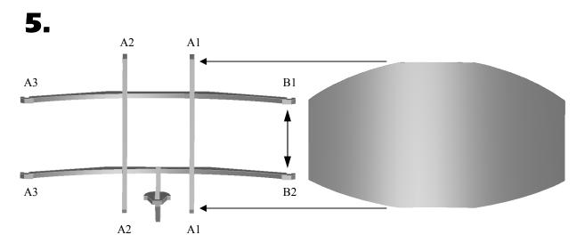
Mount the acrylic dish piece by first carefully sliding it from right to left under the retaining pieces at A1. Continue sliding left under both A2's until the leftmost edge of the dish is beneath both A3's. Then gently spread the frame at B1 and B2 until you can slide both B retainers over the rightmost edge of the dish piece.
