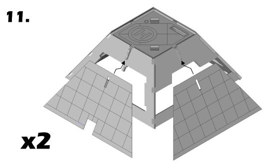
Lightly sand the back side of the 4 Acrylic sheets before installation. The sheets will fit over the MDF piece and slide up into place, slightly. Line up the sheet and then gently bend up the plastic to glue underneath.
